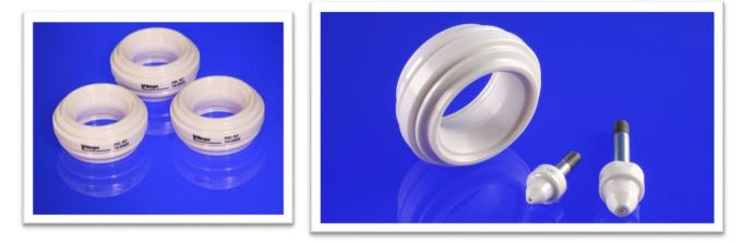
The parts are made using Nilcra Zirconia, an advanced ceramic material that is exceptionally strong and tough. It is an ideal choice for use in can production because it is highly resistant to corrosive chemicals and food stuffs but gentle on the on the internal lacquer-coated surfaces. Nilcra Zirconia is a consistent, reliable material (Weibull Modulus >30) with a low coefficient of friction. Abrasive materials have minimal effect on its surface.
